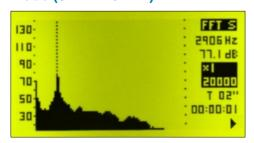
The extended frequency module of the **SC310** sound level meter adds 2 modes of measurement: Extended frequency module for 1/3 octave band analysis and FFT (Fast Fourier Transform) narrow band frequency analysis mode.
