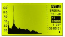
The module for vibration measurements of the **SC310** sound level meter adds 2 measurement modes; the human exposure to whole-body vibration in buildings mode and the FFT (Fast Fourier Transform) narrow band frequency analysis for vibration.
