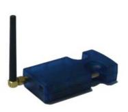
Bluetooth® Device for wireless communications for the sound level meter, BT001
